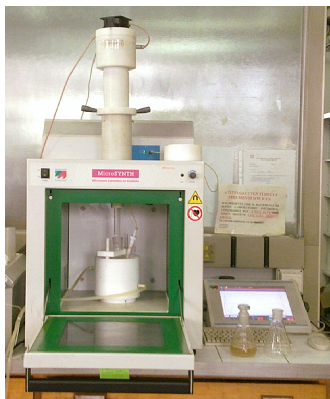
Figure 1. Combined ultrasound/microwave system with refrigerated thermostatic bath, developed at the University of Turin.
